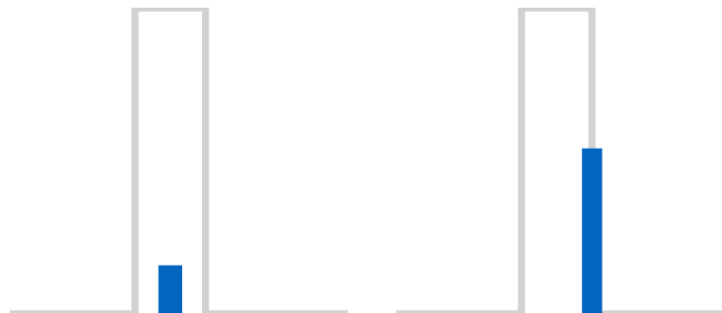
Figure 20-16 Camera-and-LED timing diagrams showing LED dimness failures: (left) LEDs are too dim; (right) LED illumination overlaps only partially with camera exposure
