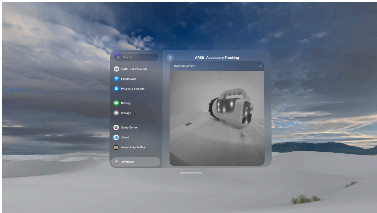
Figure 20-11 Device visual-camera view of an example accessory with well-illuminated, distinguishable LEDs ready for tracking
